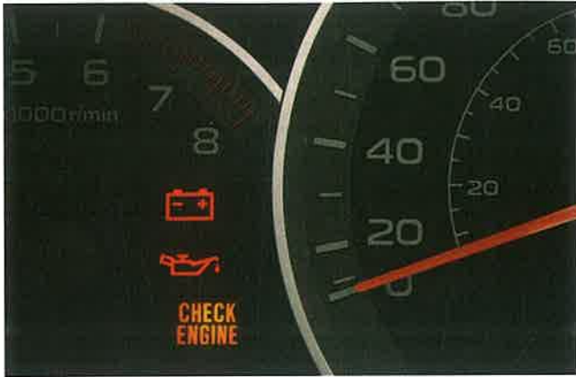
Figure 7.7: Car fault warnings.
